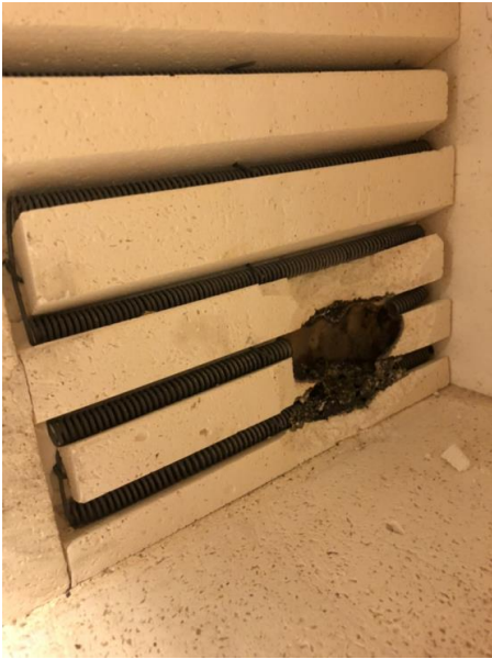
Figure 29 Damage in muffle furnace
