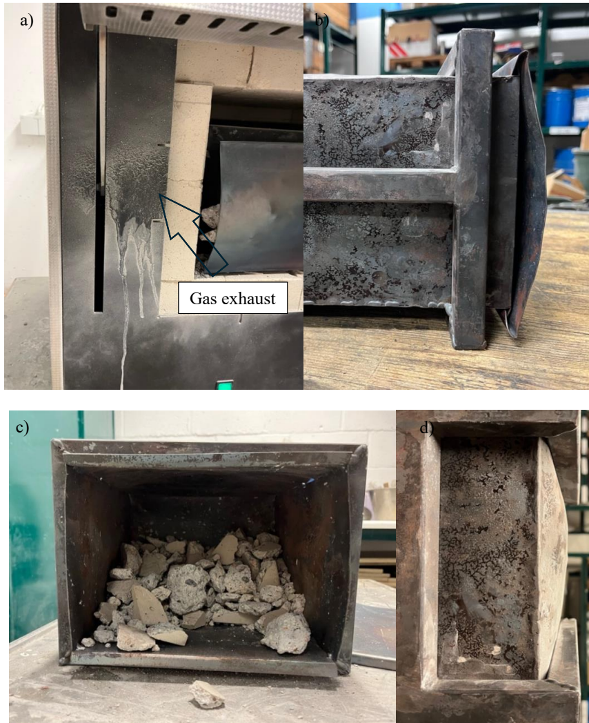
Figure 34 Metal box after explosive spalling event (a,b,c,d).
